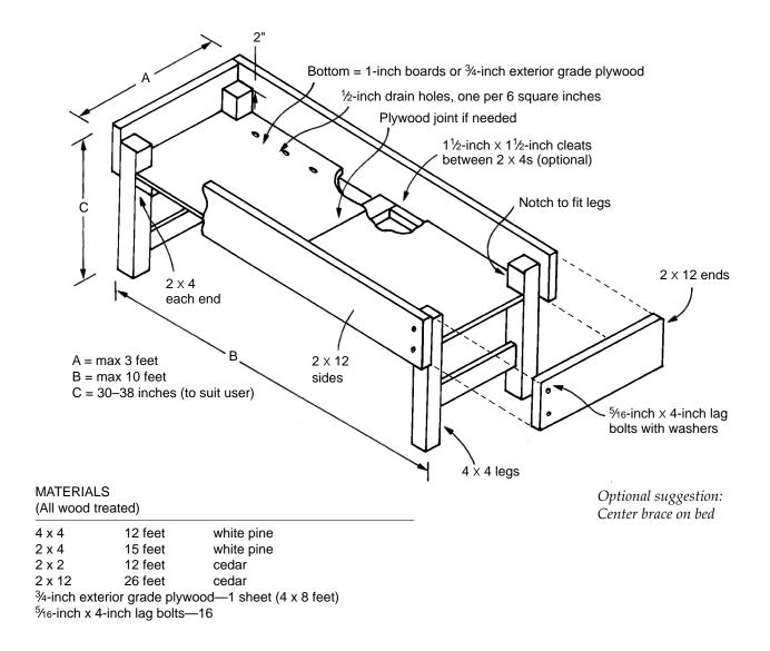
common permanent raised bed is one that has four built sides (but no built top or bottom). Usually boards and railroad ties are used to build up the bed to the desired height, but layered rocks, cinder blocks or other strong materials also can be used.
